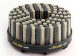
Dot Style disc brushes are used for general purpose edge deburring and surface finishing applications. The Dot style is an economical choice for light deburring applications when short cycle times are important. Dot style brushes provide greater flexibility and allow entry into small holes
